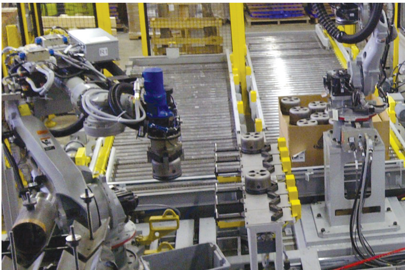
Two robots work together to pick and assemble thread protectors
